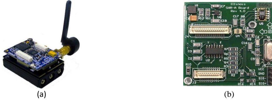
Figure 2. (a) Imote2 and (b) ISM400 sensor board.
