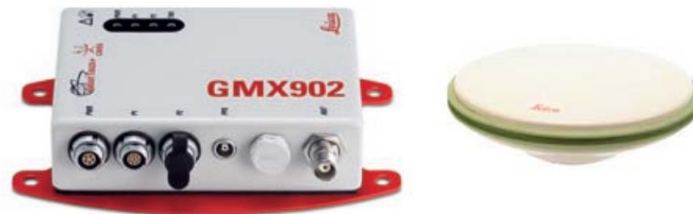
Fig. 3. Leica GMX902 dual-frequency GPS receiver (left) and AX1202 antenna (right): 0.2mm RMS accuracy, 2.4W power consumption, and up to 20Hz sampling rate (Leica 2005).
