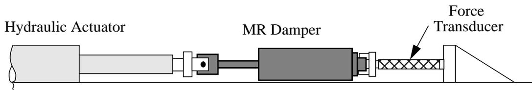
**Figure 1. Test Setup for MR Damper Identification.**
