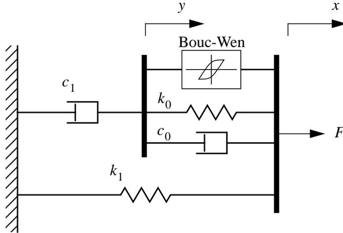
**Figure 10. Proposed Mechanical Model of the MR Damper.**
