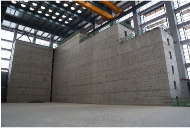
Figure 2.2 L-shape reaction wall
