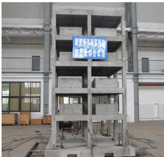
Fig. 3.1 the scale model on test of the sliding base isolation
