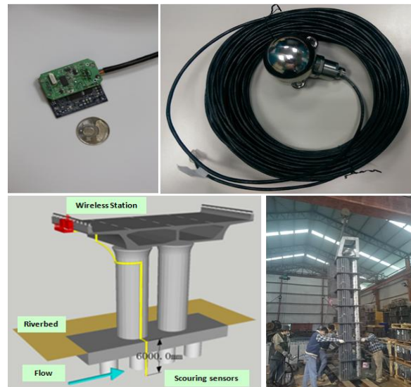
Fig. 3 Scour sensor packaged and installation
