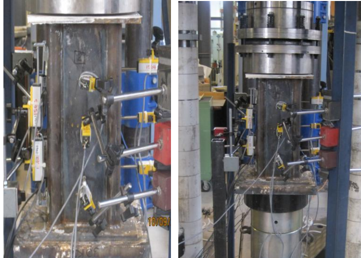
Figure 2.2 Test Set Up for Fabricated Stub Columns
