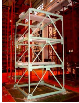
Figure 3.1 Test structure on the shake table
