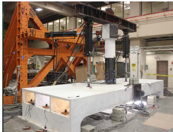
Figure 4.1 Test setup used for conducting HS trial tests for the repaired SP1
