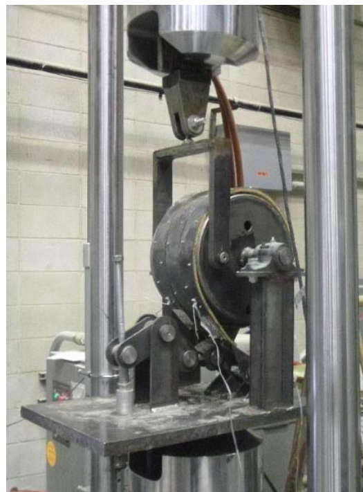
Figure 2.3 BRFD mounted in test setup
