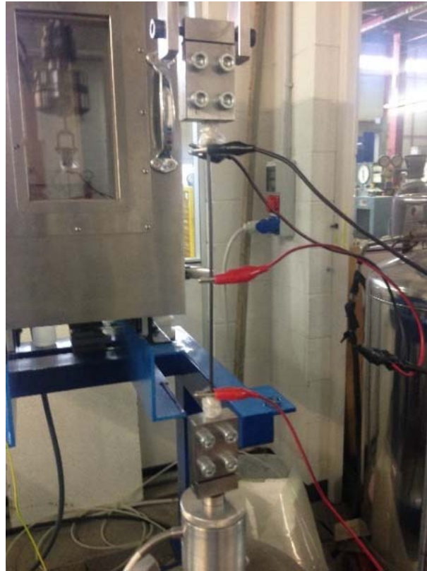
Figure 3.1 Representation of electrical resistance measurement
