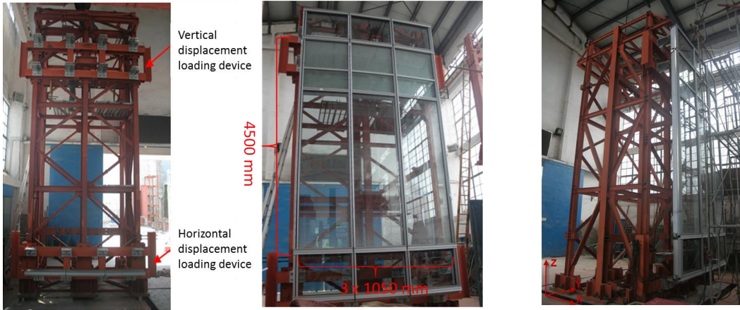
Figure 3.1 Multi-modal testing apparatus and test setup
