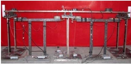
Figure 3.1 1:30 scaled highway bridge model
