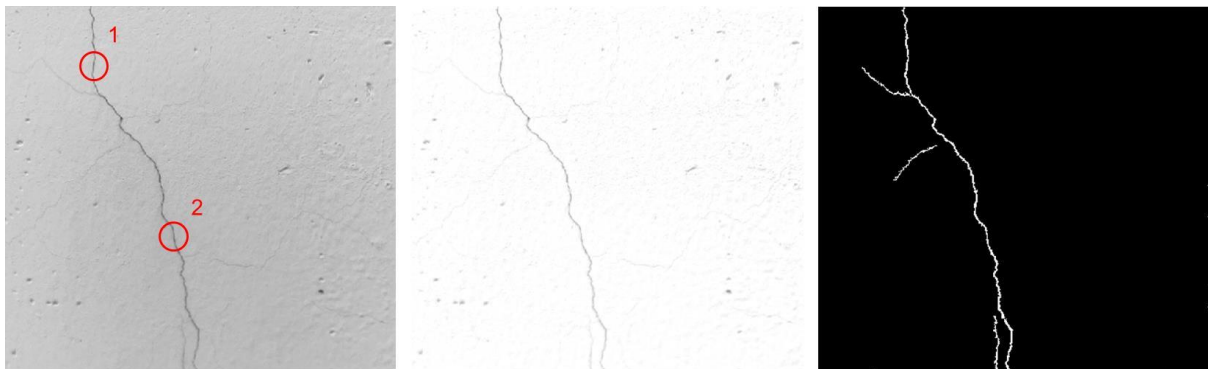
Figure 3.2 Gray-scale image, subtraction using median filter, and result of binarization and image revision
