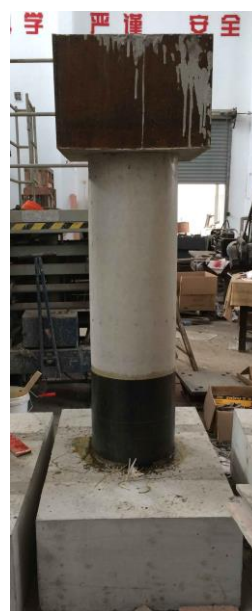
(a) Schematic of the retrofitting procedure with FRP jackets (b) Photo of a pier retrofitted with FRP jackets Figure 2.4 Schematic and photo of the retrofitting procedure with FRP jackets in the plastic hinge region of the pier
