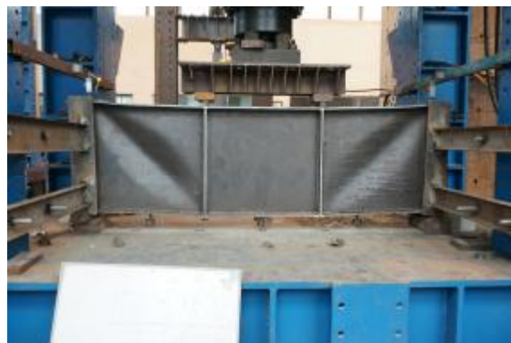
Figure 3.5 Example of local buckling (G3)
