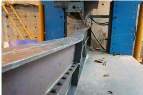
Figure 3.7 Composite beam failure (D1 for example)
