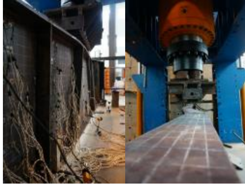
Figure 3.6 Example of lateral-torsional buckling (G4)
