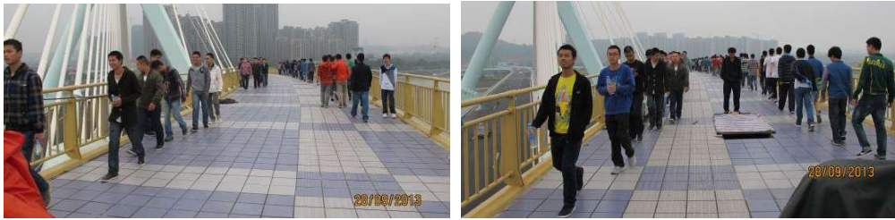
Figure 6.1 Test of the footbridge with stream of pedestrians at central span
