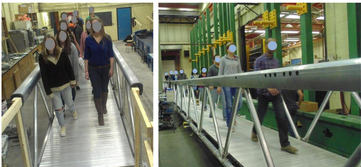
Figure 2.2 Crowd tests on the 12.2 m (left) and 22.9 m (right) bridge specimens
