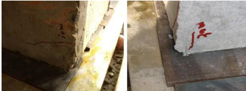
(a) horizontal crack and pastry at bottom (b) vertical crack at bottom
