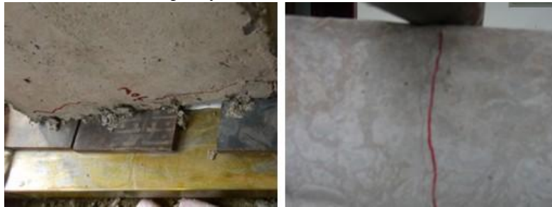
(a) horizontal crack and pastry at bottom (b) vertical crack at bottom
