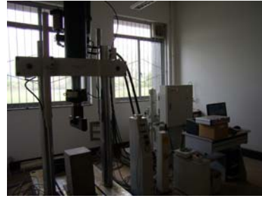
Figure 5 Shimadzu EHF-UM/UV servo-fatigue Experimental Machine
