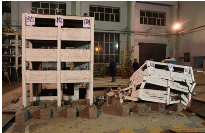
Figure 2.2 Destruction condition (Left one is model B, right one is model A)
