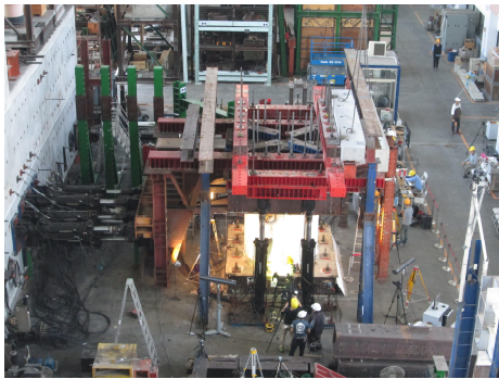
Figure 4.1 Test setup of the RCCV cyclic test
