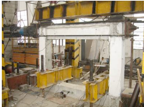
Figure 2.10 Quasi-static test for fire-damaged concrete frames
