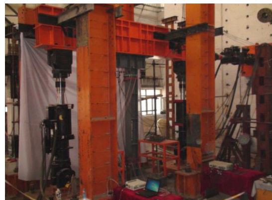
Figure 4.2 Tri-actuator Setup for experimental substructure: Column 1
