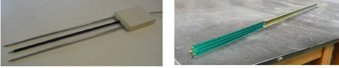
Figure 2.2 examples of TDR sensing probe (left) 3 parallel rod; (right) flexible strip scour sensor
